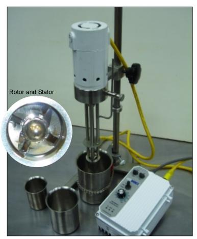
The Model CJ-2A Reversible Homogenizing Mixer was specifically designed for batch sizes as small as 250 ml. With a 1.06" diameter 12,000 RPM axial flow rotor, high shear rates approaching 50,000 reciprocal seconds are obtained. These high shear rates are capable of deagglomerating powders in liquids and emulsifying difficult immiscible liquid mixtures.
