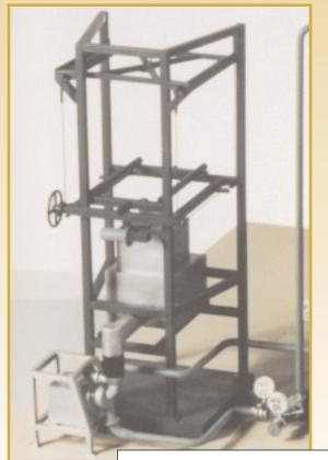
Custom Specified Systems Model D-6000 scale model with loss-in-weight feeder and individual bulk-bag handling system.
